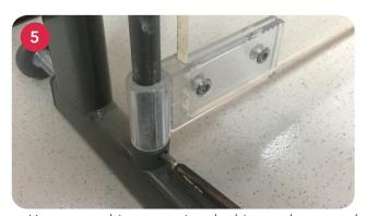
Use screw- driver screwing the hinge tube securely.
