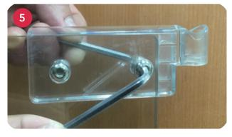
Undo the screw fixing the hinge tube and take off the corner mount. Sliding the new mount on the acrylic panel and lining up the holes. Then use the two allen key to bolt it securely.
