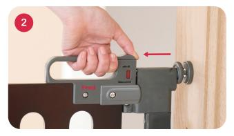
To open the Gate, holding the handle, use your thumb to slide the locking catch on the top of the Gate Panel back towards the handle, and simultaneously lift the Gate to swing it open. The window in the handle will show red when the Gate is open.
